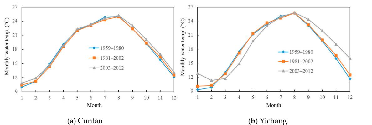
**Figure 6.** Impact of reservoirs on the monthly distribution of water temperature.
