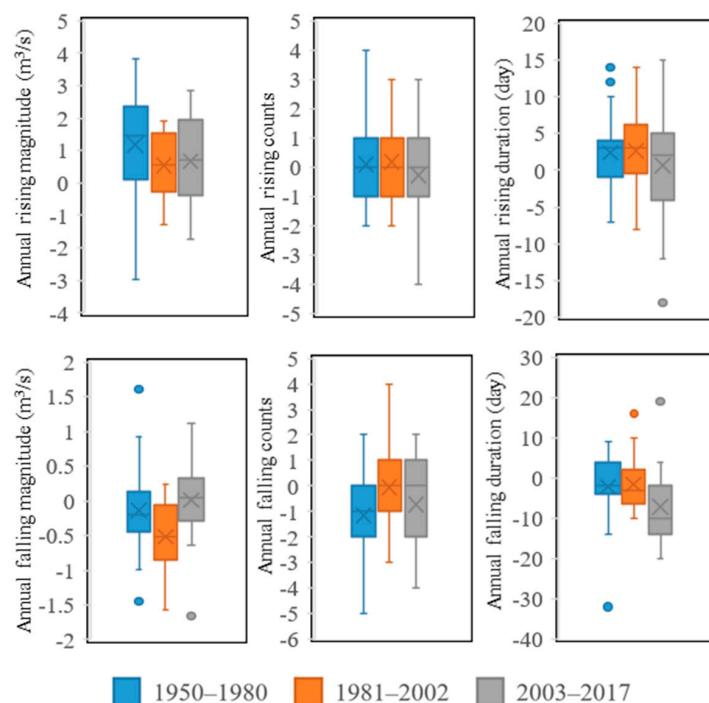
**Figure 8.** Boxplots of flow rising/falling characteristic difference between Yichang and Cuntan during May–June/October–November. The upper and lower parts of the boxes represent the 75th and 25th percentiles, respectively; the whiskers indicate the 90th and 10th percentiles; and the lines within the boxes are the median values.
